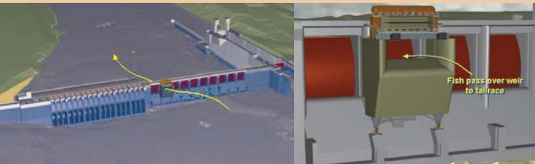
New spillway weirs attract fish close to the dam and reduce the depth they have to sound to pass over the spillway. Illustrations by Army Corps of Engineers.
